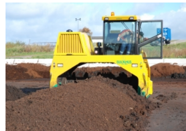
Composting of sludge in L.t.d. "Liepājas ūdens"
