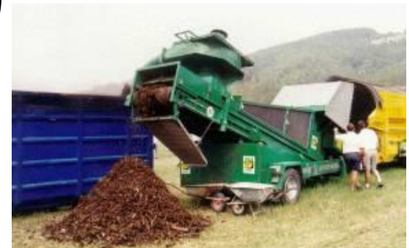
Screen; wind sifter, magnetic separator
