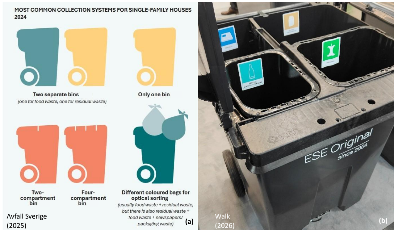
Figure 1: Applied collection container configurations in Sweden 1 and example of four-compartment bin
